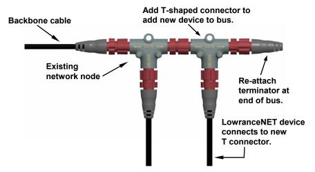
Add a new device to a NMEA 2000 bus by attaching a T connector between two T connectors, between a T connector and the end terminator, or between two backbone extension cables.
