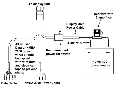
Use this method if you are *only* powering your display unit and are not powering a NMEA 2000 network or any NMEA 2000 accessory device, including a GPS module.
